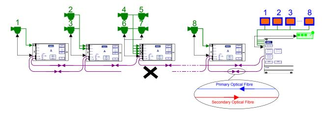
If multiple breaks occur, operation is maintained will all the units still physically connected to the receiver. For the scenario shown below camera signals and control would now be lost from cameras 1,2 and 3 as there is now no physical connection between the transceivers and the receiver. However operation of cameras 4,5,6,7 and 8 remains fully functional.
