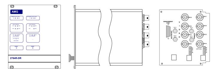
**AMG2784R-DR** is a rackmount eight channel video receive unit designed to 'drop off' eight video signals from a dual fibre optical fibre ring. It also provides a single RS485/RS422 or RS232 bi-directional data channel to the video insert outstations. The **AMG2784R-DR** is designed to plug into an **AMG2000** or an **AMG2005** subrack which in turn fits into a 19" rack system.
