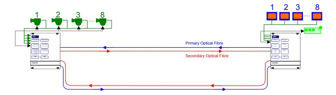
Again if one of the routes is broken, operation of the system is maintained as shown below:
